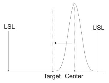
If Cp is less than Cpk (data is centered but does not fit between the spec limits.) the corrective action is to improve the process to eliminate non-conforming parts:
