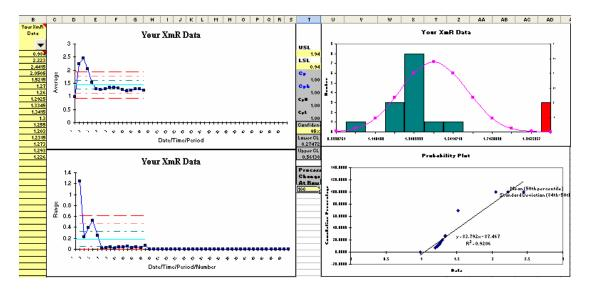
Since you're starting in cell B2, Wedgelink will type the data followed by a carriage return (CR) which moves the cursor to cell B3 and so on. As you press the data button on the gage, the spreadsheet fills with data and the control charts, histograms and normal probability plot update *automatically*!
